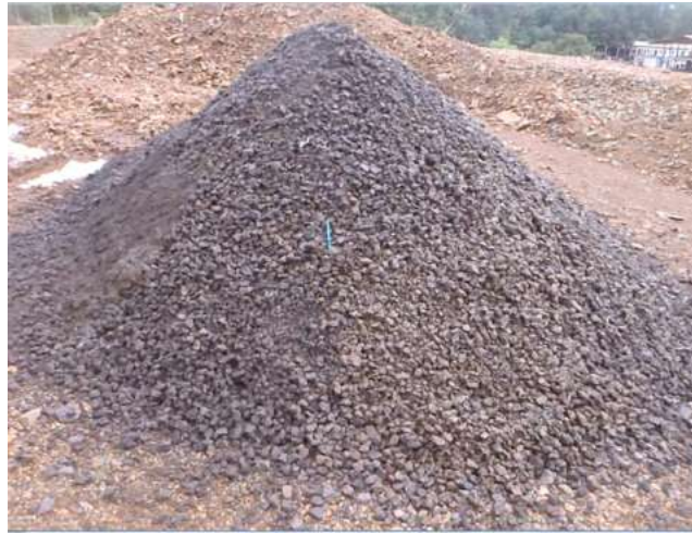
Figure 2 Nickel slag coarse aggregates after processing
