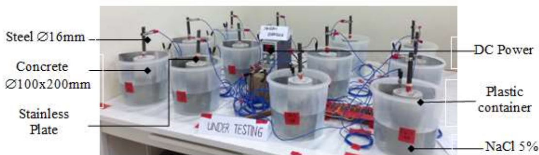
Figure 3 Corrosion acceleration setup in the laboratory
